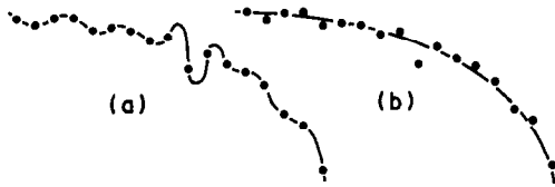
Fig. 1. Examples of the approximative spline function (a) and rational spline function (b) fitted to the same set of points.
